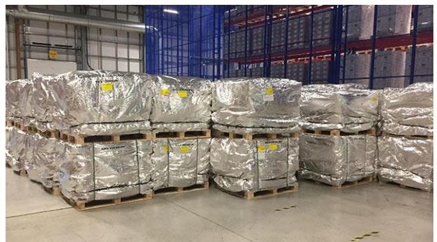
Pallets of finished pharmaceutical product wrapped in passive thermal covers
